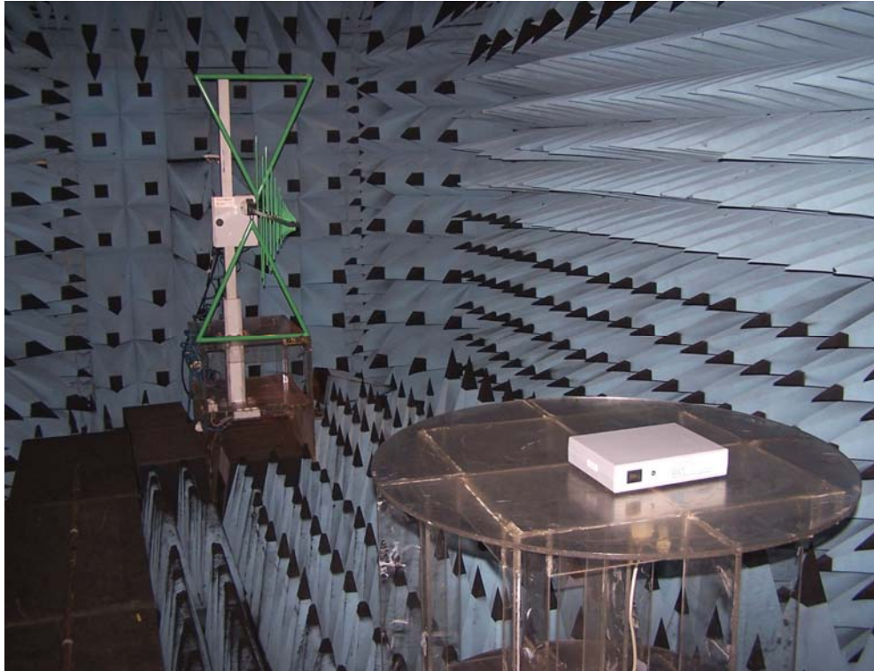
Photo 1: Test setup in the anechoic chamber, radiated emission measurements
