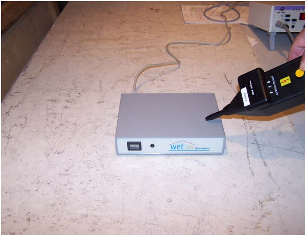
Photo 6: Test setup in the shielded high frequency laboratory 1, Electrostatic discharge immunity tests
