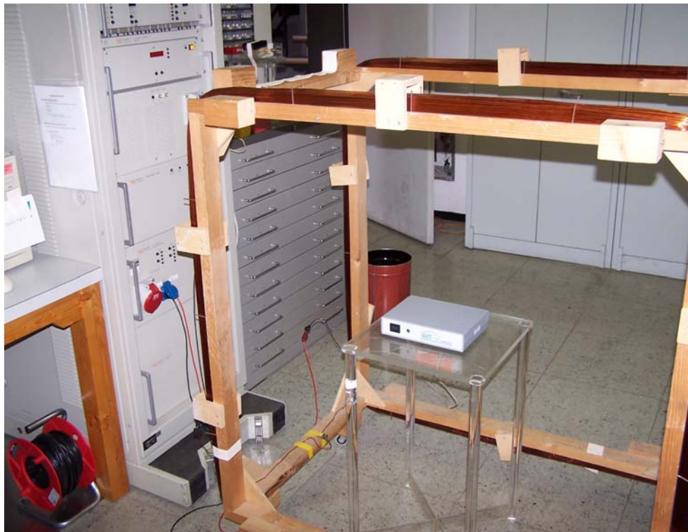
Photo 8: Test setup in the laboratory 2, power-frequency magnetic field immunity tests
