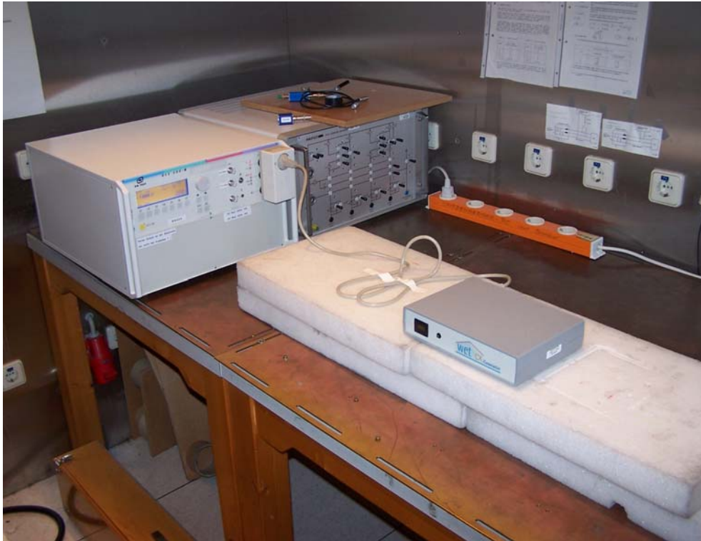
Photo 5: Test setup in the shielded high frequency laboratory 1, Burst and Surge immunity tests
