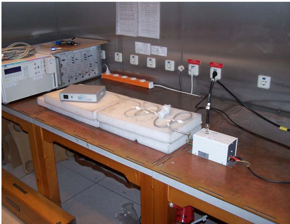
Photo 4: Test setup in the shielded high frequency laboratory 1, Radio-frequency continuous conducted immunity tests
