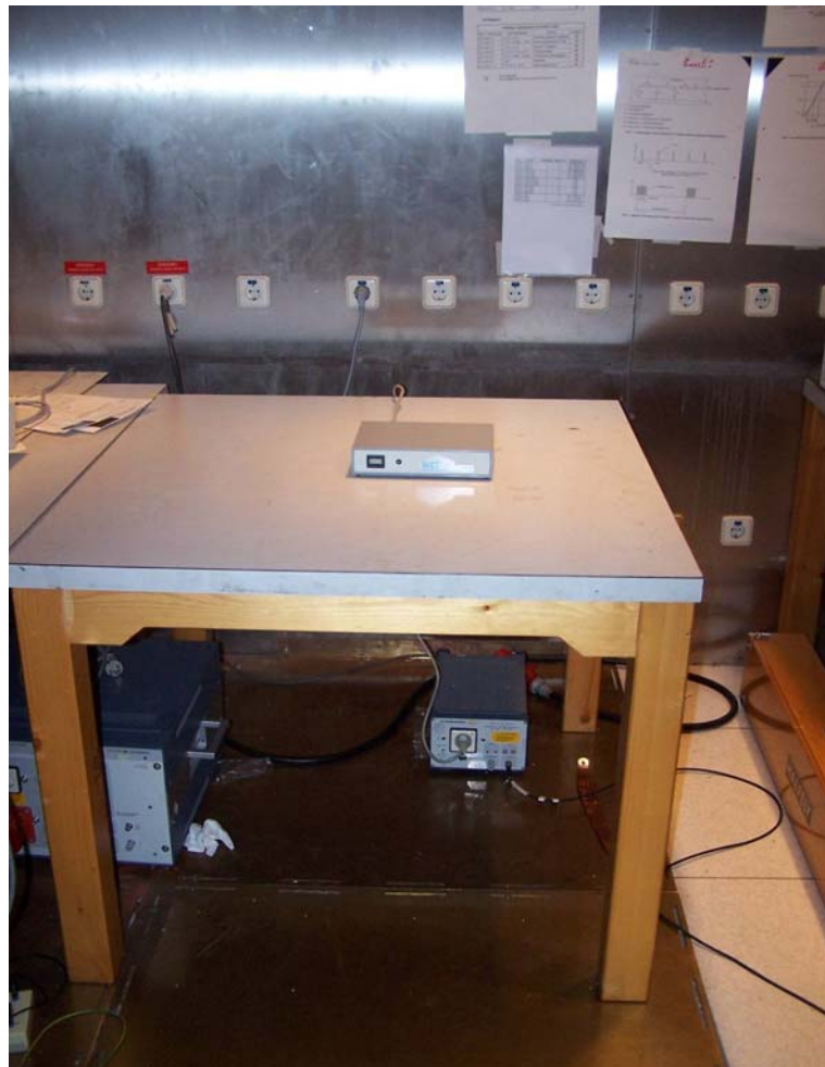
Photo 2: Test setup in the shielded high frequency laboratory 1, conducted emission measurements
