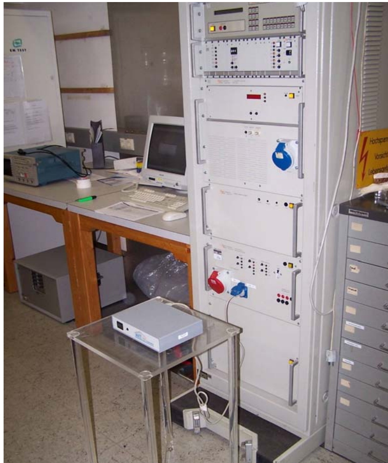
Photo 7: Test setup in the laboratory 2, voltage dips and interruptions immunity tests, harmonic current emissions and flicker measurements
